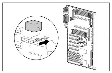
Figure 2-39. Installing the external replacement battery
